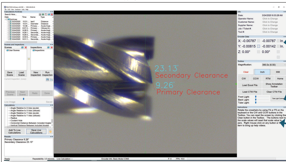
Primary and Secondary Clearance Angle at 390X zoom
