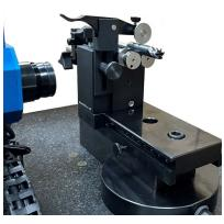
The PG concentricity fixture, also known as a 3 roller, provides a constant smooth part rotation that allows for easy and accurate measurements of the tool. All precision concentricity fixture are certified to be accurate within  $2\mu$  over the rollers. Each
