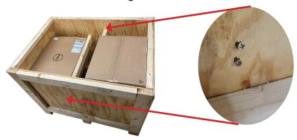
Remove lag bolts with 9/16" socket driver. When lifting/removing the  $2\times4$  securing the PG1000 unit to the crate, **be very careful not to hit the**
