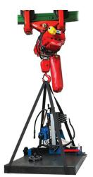
Do not turn the handwheels until the (3) locking bolts and (1) locking bar are removed or damage will occur.
